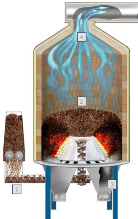
Updraft Gasifier: 1. Fuel Source 2. Roasting Cham-ber 3. Ash Bins
