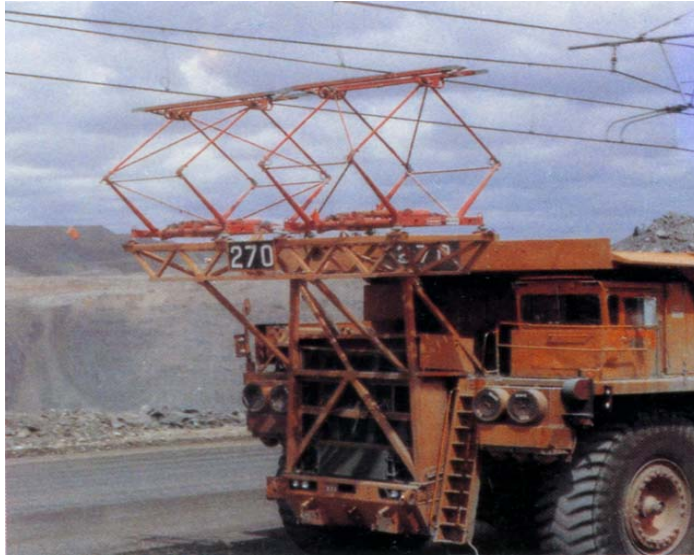
Open Pit Haul Truck with Trolley Power Cantilever
